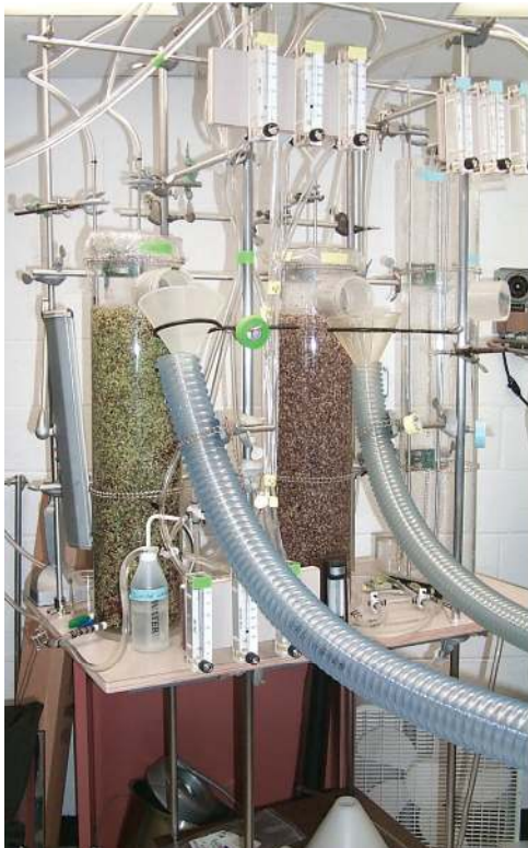
The hydrosprouter that Dr. Fahey invented as a result of trying to optimize sprouting in his lab.
